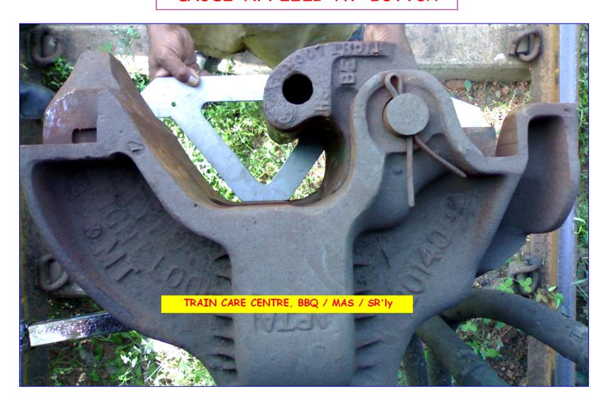
Description: The gauge must seat against the front face of the coupler head and the pivot lug and clear at all points around the interlocking lug guard arm face and lateral aligning surface.
