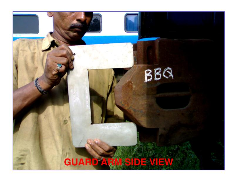
Description: The gauge must not pass into the wing pocket or over the guard arm.
