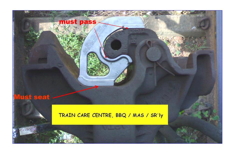
Description: This gauge must pass through the contour with the knuckle fully closed and locked.
